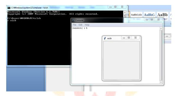
Therefore, wish provides an interactive prompt from which you can enter Tk commands to create a graphical interface. As wish interprets the commands, it displays the resulting graphical interface in the window.
